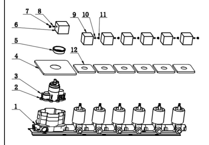
Before install No 3, open the piping switch to counter flush and clean any debris in the pipes, please note the hot and cold sign.
